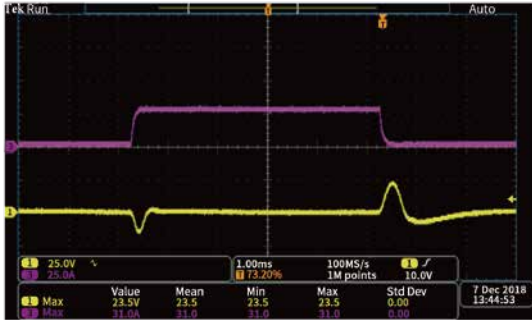
Standalone unit IT6006B-500-40 500V 40A 6000W Setting: voltage 100V current 28A Load current: 30A
